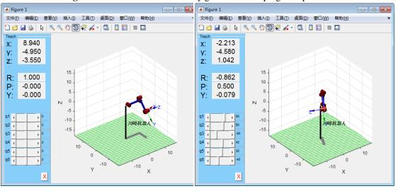
Figure 7: Pose matrix of robot body generated after program operation
