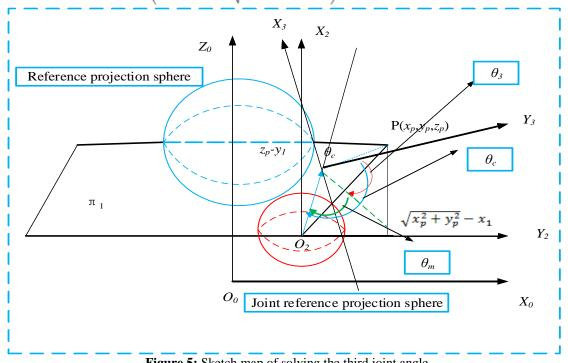
Figure 5: Sketch map of solving the third joint angle
