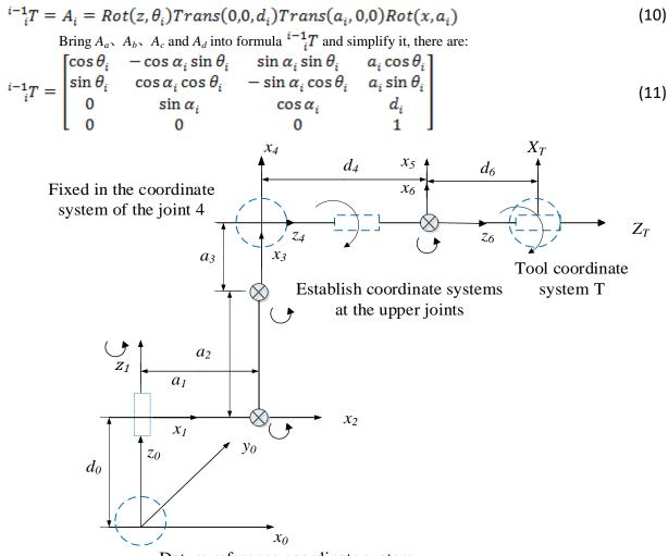
Datum reference coordinate system **Figure 1:** Sketch map of robot body kinematics coordinate system
