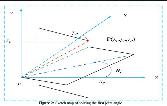
According to the actual situation of the problem, Formula 17 equal value principle on both sides of an equal sign, Because  $(x_p, y_p)$  is known, Combining the projective geometric meaning of  $\theta_1$  in figure 2, The first joint angle  $\theta_1$  can be obtained, there are:
