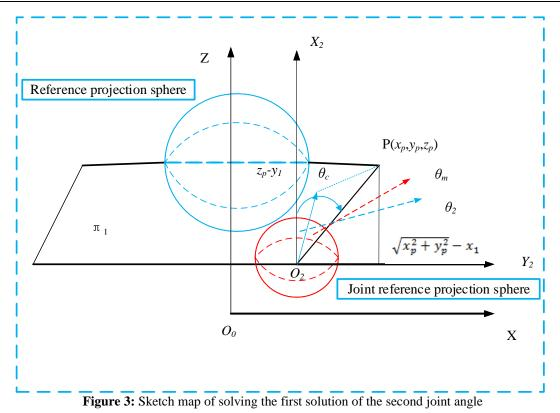
By analyzing the geometric meaning of  $\theta_2$  and the valid range of  $\theta_2$ ,  $\theta_2$  has two values, refer to the projective geometric meaning of figure 4, and further simplify, we can get another solution of  $\theta_2$ , there are:
